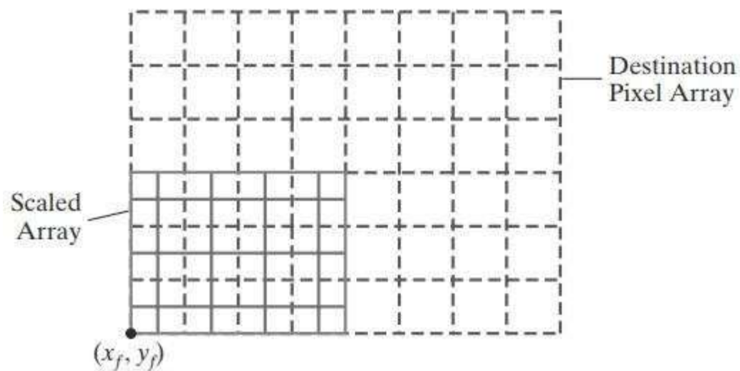
Figure 2.23: Mapping destination pixel areas onto a scaled array of pixel values. Scaling factors s_x = s_y = 0.5 are applied relative to fixed point (x_f, y_f) .
